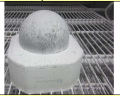
Test for protection against solid foreign objects (Dust test)
